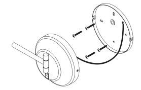
6. Connect the electrical wires coming from the electrical box to the terminal connections. Tighten the set screws.
